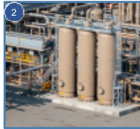
2 MOLECULAR SIEVE DEHYDRATION Used to remove water from natural gas.
