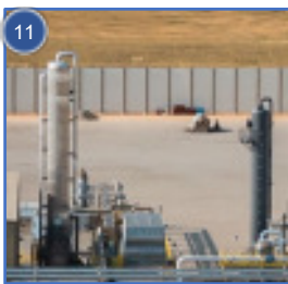
11 AMINE TREATING Removes Carbon Dioxide from the inlet gas stream.
